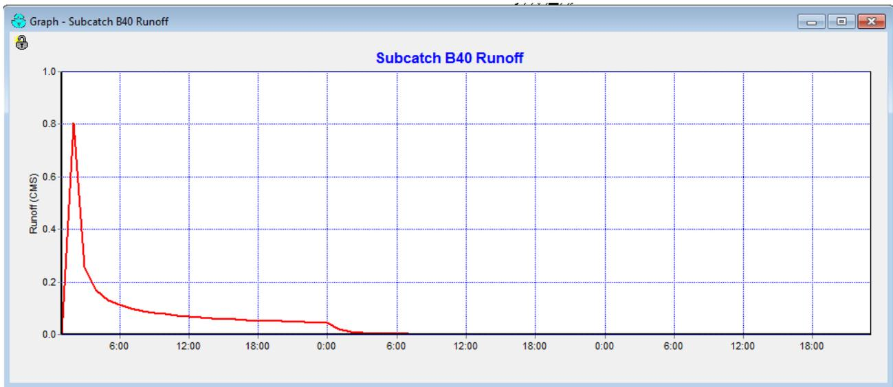
**Figure 4.** The peak flood discharge diagram in the hydrological unit 40 obtained from the SWMM software 4-1 - Evaluation of the transfer capacity of conduits
